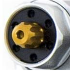
C1: Adjustable compression damping. Gold adjuster on TTX36 / TTX GP shocks.
