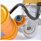
C2: Adjustable high and low speed compression damping on S46 shocks. Hexagon and slot on the reservoir.
