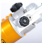
C1: Adjustable compression damping. Adjuster wheel or slot on the reservoir.
