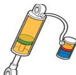
H: Monotube high pressure gas type of shock absorber with hose mounted external reservoir.
