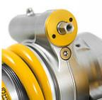
B: Integrated hydraulic spring preload adjuster. Adjuster wheel or hexagon on the adjuster.
