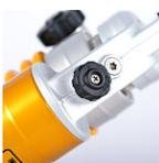
C1: Adjustable compression damping. Adjuster wheel or slot on the reservoir.
