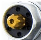
C1: Adjustable compression damping. Gold adjuster on TTX36 / TTX GP shocks.
