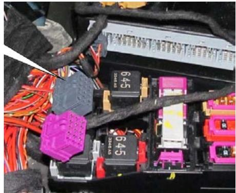
Fix the control box with hook-and-loop tape.
