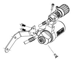
Install the shock absorber with the hose connections down and hoses to the left side of the bike. Install the rear shock absorber attachment first.
