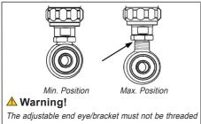
out more than that the groove is fully visible beneath the lock nut. This is maximum length. After adjusting, make sure that the lock nut is tightened (30Nm).
