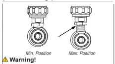
The adjustable end eye/bracket must not be threaded out more than that the groove is fully visible beneath the ock nut. This is maximum length. After adjusting, make sure that the lock nut is tightened (30Nm).
