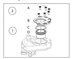
Put the motorcycle on a workstand. Remove the front fork and triple clamps. Remove original upper steering stem nut and washer (you will not need these parts to install the Öhlins steering damper).
