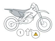
Put the motorcycle on a workstand so that the rear wheel barely touches the ground.
