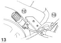
Fix the adjuster and let the hose go in soft turns to the spring pre loader. Fix the hose with tie-raps.
