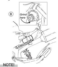
It might be necessary to modify the attachment slightly by grinding the rear edge so the adjuster wheel not will be in contact with the edge.
