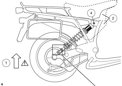
Remove the upper attachment and remove the original shock absorber.
