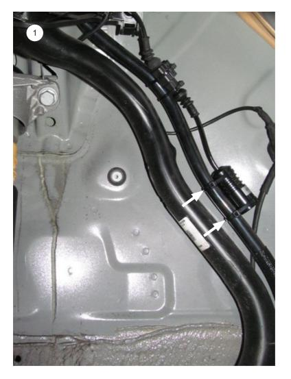
Fix the wire of the electronic component with cable ties.
