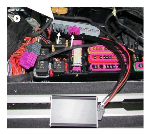
Fix the control box with hook-and-loop tape.
