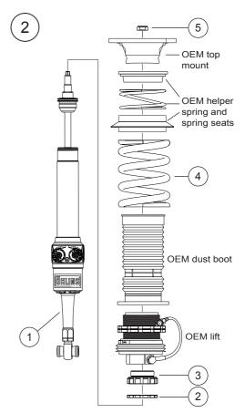
Tighten the OEM lifter against the lift adapter (2) to 50-60Nm. Tighten the lock ring (3) to 50-60Nm. Continue installing the OEM dust boot, the main spring (4), the OEM helper spring and upper spring seat. Snap the OEM dust boot in place on the OEM upper spring seat and install the OEM top mount and the lock nut (6). Tighten the lock nut to 35-40 Nm.
