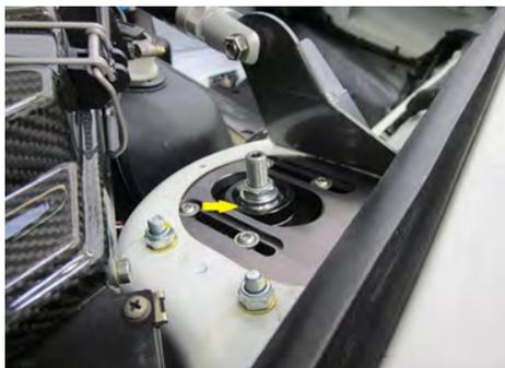
Fig.4 Camber adjustment top mount
