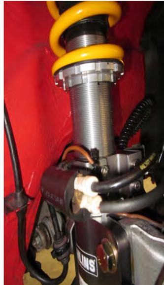
Fig.2 Damper mounted to wheels mounts
