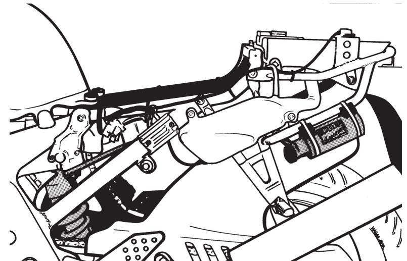
On this model is an adjustable end eye/ bracket mounted. The end eye/bracket must not be threaded out more than that the groove is visible beneath the locknut. See fig. Make sure that the locknut is tightened after adjustment.
