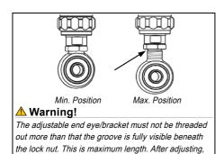
make sure that the lock nut is tightened (30Nm).
