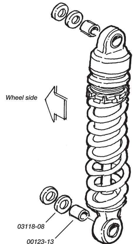
*Normally the shock absorber is mounted with the cylinder head upwards. Check that there is enough clearance to other details both in loaded and unloaded position.*
