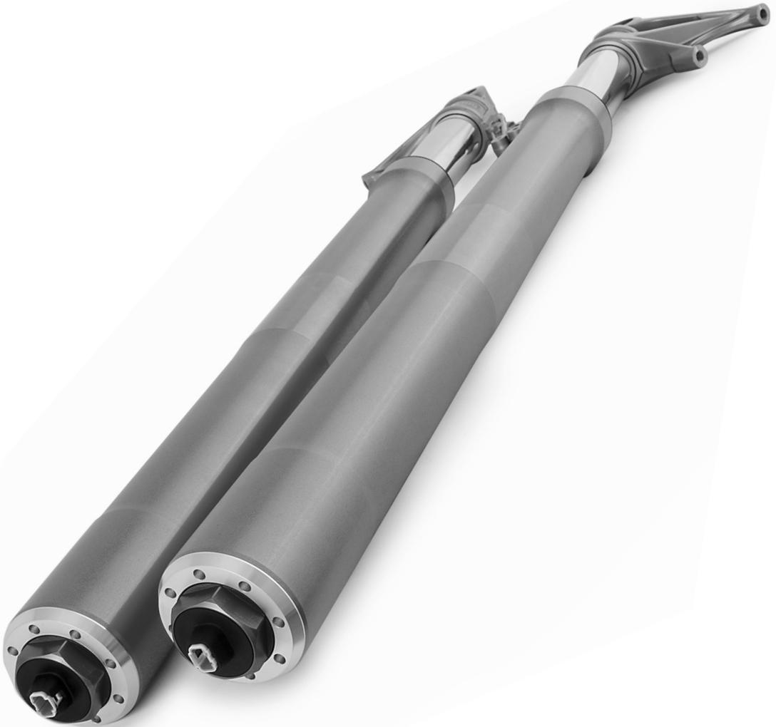
When adjusting the spring preload you move the spring seat. This will decrease or increase the initial spring force, which will lower or raise the motorcycle rear ride height.
